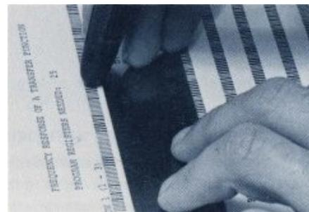
Where **nn** is the number of the next bar code row to be scanned. If the HP-41C sounds the scan error tone while you are scanning program bar code, refer to [appendix A](#), Errors and Messages.
