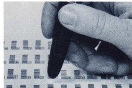
2. Press the recessed scan switch and lightly place the wand tip on the paper. The tip should be placed about 1 cm (approx. 0.4 in.) from the first bar in the row.
