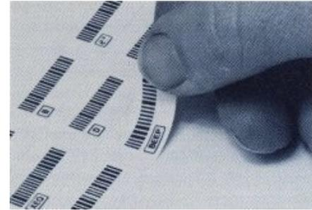
One of the protective transparent sheets you received with the wand should be placed over any set of labels you are going to scan. The transparent sheet will protect the labels and reduce the possibility of the wand reading label edges as bars and causing an error condition.
